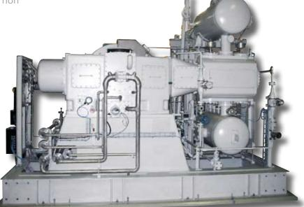
High speed 400 kW block for gas turbine feeding in Lithuania up to 1,000 psi [70 bar]. Variable speed to control the flow according the need of the gas turbine system.
