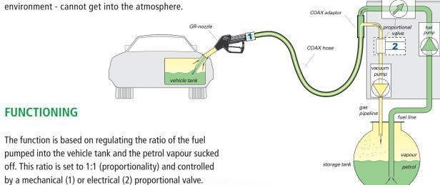
Legal requirements and automatic monitoring systems place the highest demands on the reliability of vapour recovery systems. In case of a problem with the vapour recovery the filling station operator is required by law to switch off the petrol pump within a certain limited period of time. In Germany this period is 72 hours.
